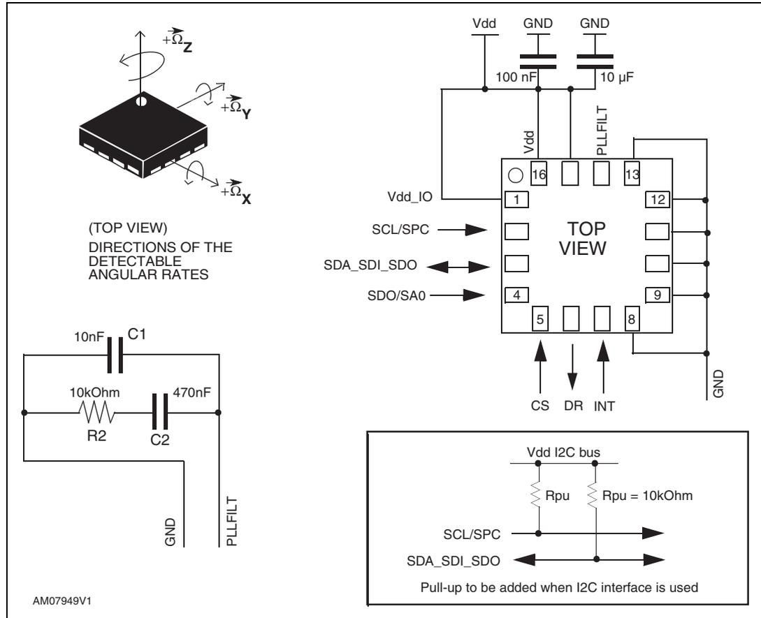
Power supply decoupling capacitors (100 nF ceramic or polyester +10 μF) should be placed as near as possible to the device (common design practice).
