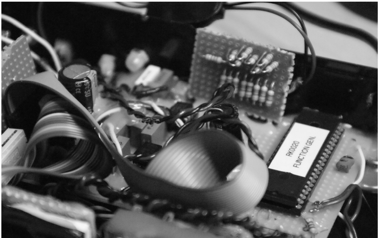
Picture 3.2 – Close up view including R/2R resistor DAC
