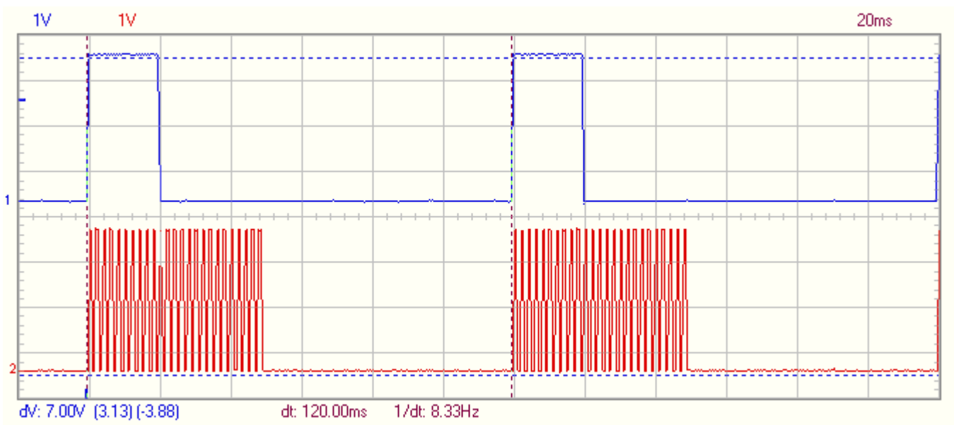
Figure 2: DelayedOut_bit (blue) and LedOut_bit (red)
