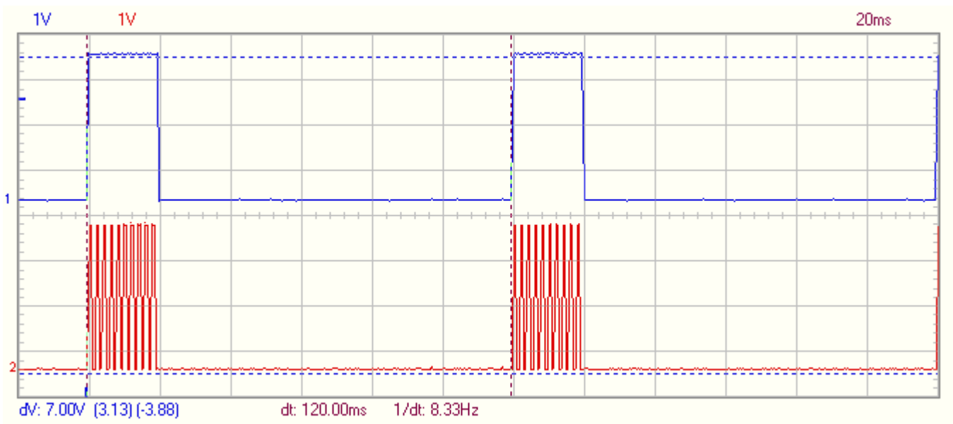
Figure 1: DelayedOut_bit (blue) and OscOut_bit (red)
