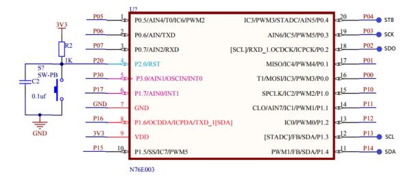
\*Note that the pin naming of the chip in the schematic above is wrong. P13 and P14 are both SDA pins according to this naming when actually P13 is SCL and P14 is SDA pin.
