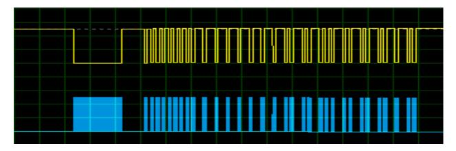
In this segment, we will see how we can use an external interrupt and a timer to easily decode a NEC IR remote. This same method can be applied to any IR remote controller. At this stage, I recommend that you do a study of NEC IR protocol from <u>here</u>. SB-Project's website is an excellent page for info as such.
