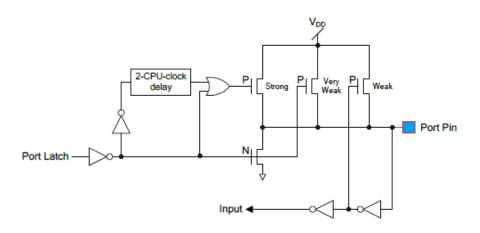
On close inspection, we can realize that this structure has striking resemblance with the GPIO structure of a typical 8051 microcontroller as shown below:
