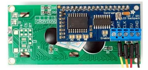
In this segment, we will be driving a 2x16 LCD with CD4094B Serial-In-Parallel-Out (SIPO) shift register using software SPI. The same idea can be used for other similar shift registers like 74HC595. There are other ways of using SPI-based LCDs but the aforementioned are the cheapest ways.
