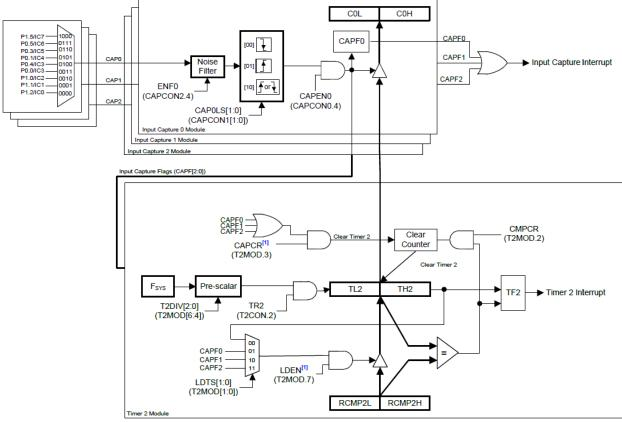
[1] Once CAPCR and LDEN are both set, an input capture event only clears TH2 and TL2 without reloading RCMP2H and RCMP2L contents.
