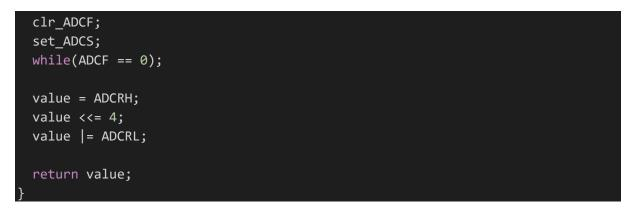
When this function is called, the ADC conversion completion flag is cleared and the ADC is softwaretriggered. The conversion completion flag is polled. When this flag status is changed, the ADC data registers are read. Finally, the value is returned.
