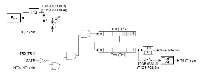
Check the block diagram shown above and compare with the one previously shown. Note the greyedout part in this diagram. The upper bits of TL registers are not used in this mode. Between Mode 0 and 1, personally Mode 1 is easier than Mode 0.
