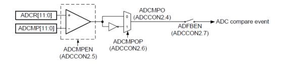
The comparator block is situated at the output of the ADC and so it is just a single block like the ADC but all eight channels share it. Thus, when it is needed to compare multiple channels, it should be reset and reconfigured.
