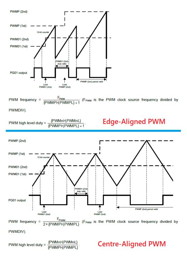
The first type was demonstrated in the simple PWM example. The second is demonstrated here. From the perspective of a general user, the difference in them don't affect much. Make sure that you check the formulae for each type before using.
