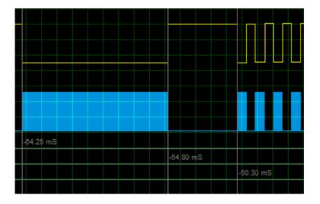
Logic one is represented by a pulse of 560 $\mu$ s high time and 2.25ms of low time – total pulse time is 2.81ms. Likewise, logic zero is represented by a pulse of 560 $\mu$ s high time and 1.12ms of low time – total pulse time is 1.68ms.
