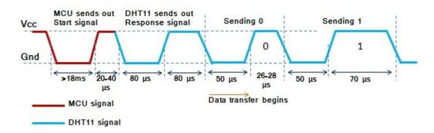
Shown above is the timing diagram for DHT11's time slots. Check the length of pulse high time for one and zero. This is the technique applied in time-slotting mechanism. We have to time pulse lengths in order to identify the logic states.
