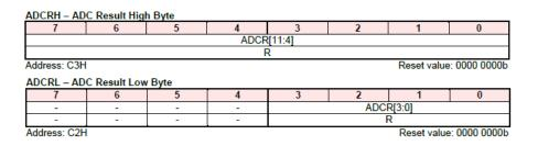
Notice that the we must extract ADC from **ADCCRH** and from the low four bits of **ADCCRL**. To handle this issue the follow function is devised:
