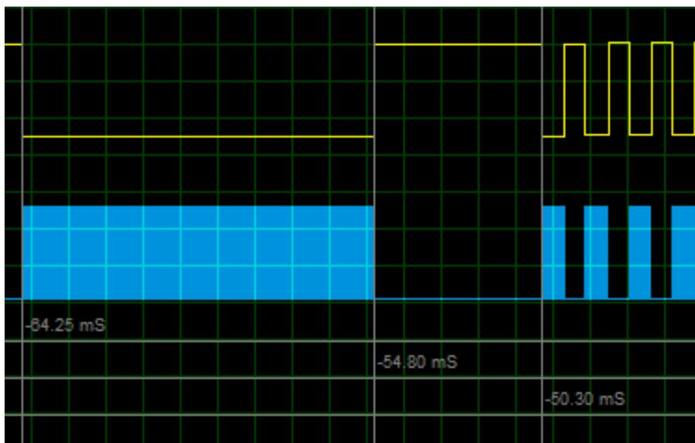
Logic one is represented by a pulse of 560µs high time and 2.25ms of low time – the total pulse time is 2.81ms. Likewise, logic zero is represented by a pulse of 560µs high time and 1.12ms of low time – the total pulse time is 1.68ms.
