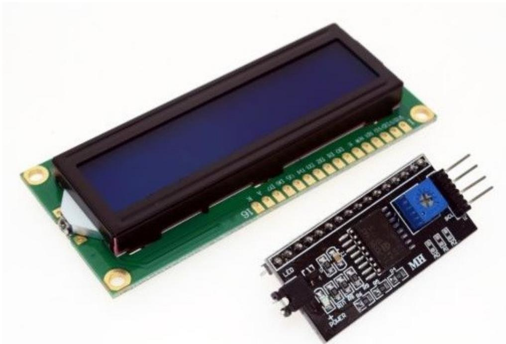
The demo for this example is a simple multi-UART chatting. One UART is hardware-based while the other is based on software. The chatting between the UARTs is displayed on I2C-based serial LCD. This LCD is driven using I2C-based PCF8574 GPIO expander.
