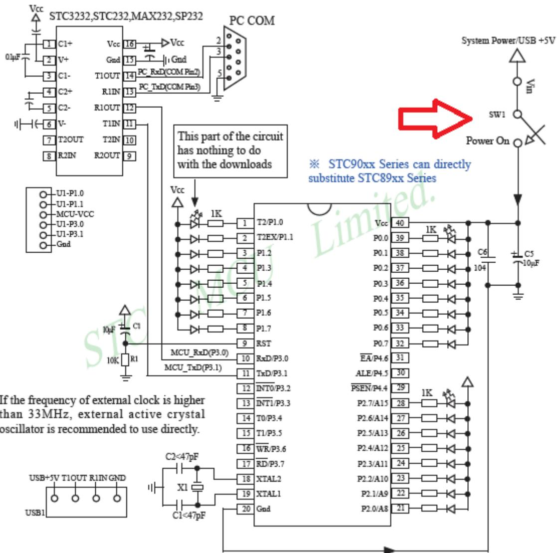
This is why the red arrow highlights the power switch in the schematic. Though the schematic shows a MAX232-based converter, we can use a USB-serial converter instead.
