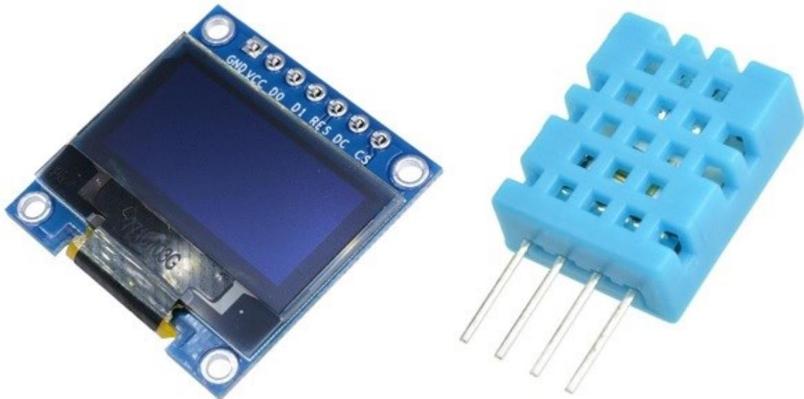
Likewise, bit-banging can also be applied to communicate with one wire devices such as DHT11, DHT22, etc.
