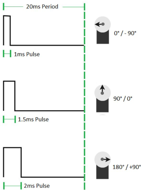
Each pulse has a period of 20ms but the duty cycle/pulse high time is varied from 5 - 10% to rotate from one direction to the other. This clearly demonstrates why timing is very important for servo motors.
