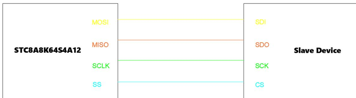
Since SPI bus is very fast, it is widely used for interfacing displays, flash memories, etc. that needs fast responsiveness.
