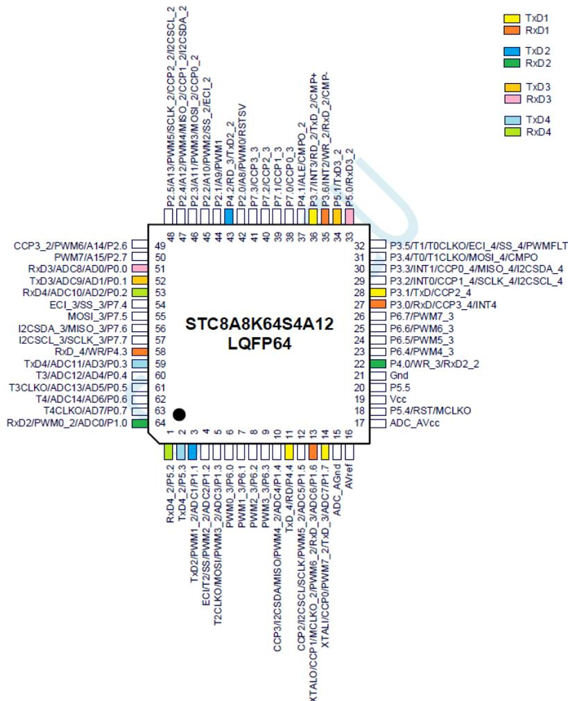
I2C hardware available in STC8A8K64S4A12 is very simple but it offers lot of flexibilities. The I2C block can be used in both I2C master or slave roles. Just like UART it has lot of alternative pin pair options as the table below shows.
