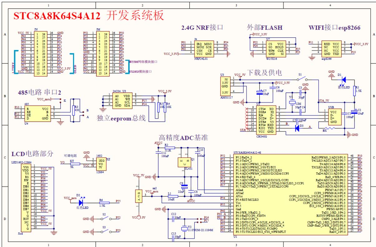
On board, we have connectors for OLED display, GLCD, LCD, TFT Display, nRF24L01 transceiver, ESP8266 Wi-Fi module, etc. We also have on board W25x16 flash, 24C04 EEPROM, RS485 communication bridge and a CH340G USB-serial converter that doubles as an on-board programmer.
