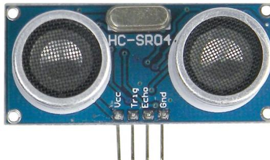
There are two pins apart from the power supply pins and these are needed to communicate with the sensor. When the trigger pin of the sensor is pulled high for about 10μs, the sensor acknowledges this short duration pulse as a command from its host micro to measure and return range data. A pulse output from the echo pin is the representation of distance.
