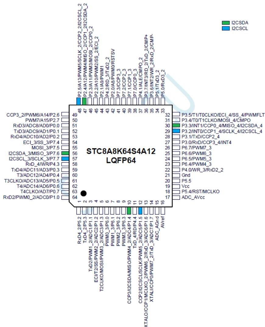
SPI hardware is also fully implemented in STC8A8K64S4A12. Using the SPI hardware is very simple and like other communication peripherals, we have options to use various alternative GPIO pin groups. Both SPI and I2C blocks are fully independent blocks unlike UARTs as UART blocks are dependent on internal hardware timers.
