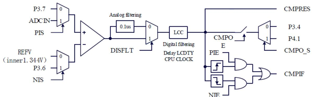
The comparator block shows that P3.6 and P3.7 GPIO pins can be used as positive and negative inputs to the comparator unit. Alternatively, we can also use internal 1.344V voltage reference source or ADC input. The comparator output can be optionally filtered both using analogue and digital techniques. Lastly, we can retrieve comparator output via GPIO pins, flag and interrupts.
