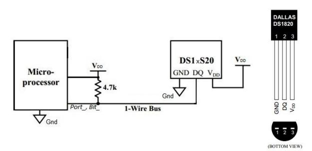
As one can see there is, besides the actual "1-wire bus" connection, only need for pull-up resistor of 4.7K plus a ground and a Vdd connection to the Ds18x20. The latter is called "External Power" in the datasheets (see section 7.3). The Vdd connection can by avoided by using the <u>parasite Power</u> possibility, see section 6.1.
