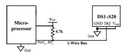
The only issue here is that the DS18x20 consumes a rather high current during temperature conversion, which is not possible via the pull up resistor. To ensure that the device gets enough power via the 1-wire bus the PIC must pull that line high during the whole temperature conversion time.
